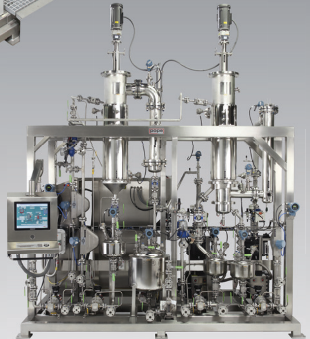
Two-Stage 12" Production Scale Cannabinoid Distillation System For Up To 60 kg/hr
